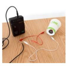
Plug the mini phone plug into your radio, phone or other device, then turn it on and play some music (you may have to turn the volume up louder than you normally would). With one hand, hold the cup to your ear. With your other hand, bring a magnet closer and closer to the coil of wire until you can hear the sound produced by your homemade speaker.
