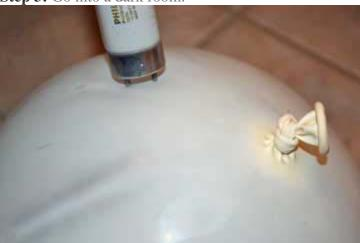
**Step 4:** Touch the balloon against the two metal electrode prongs on the bottom of the fluorescent light bulb.
